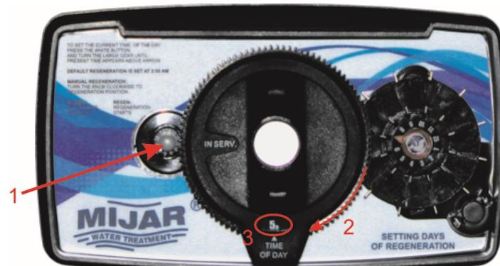
To set the current time, the user must press and hold the white button (1), and simultaneously turn the gearwheel (2) so in the gap (3) the current time is shown\* (like on the watch). Next, release the white button (1) so it falls back between the gearwheel pins.
